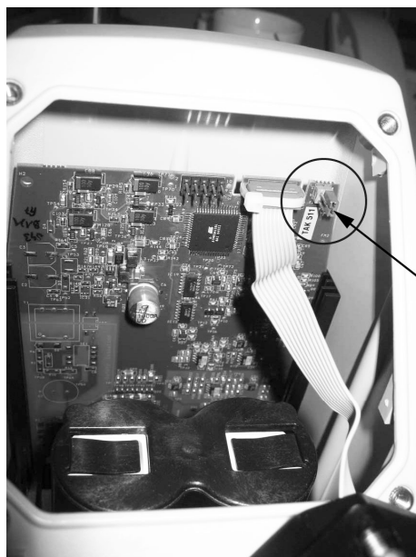
Figure 7-5 HW key behind the display (placed on the right pins)
